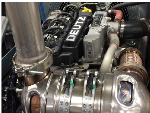
DEUTZ DOC, Diesel Oxidation Catalyst; allows for maintenance free operation
