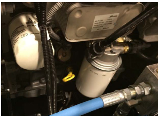
Easy Access fuel filter, oil filter and dipstick
